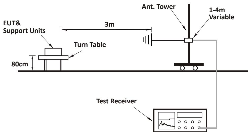
**TEST REPORT****For Radiated emission above 1GHz:**
