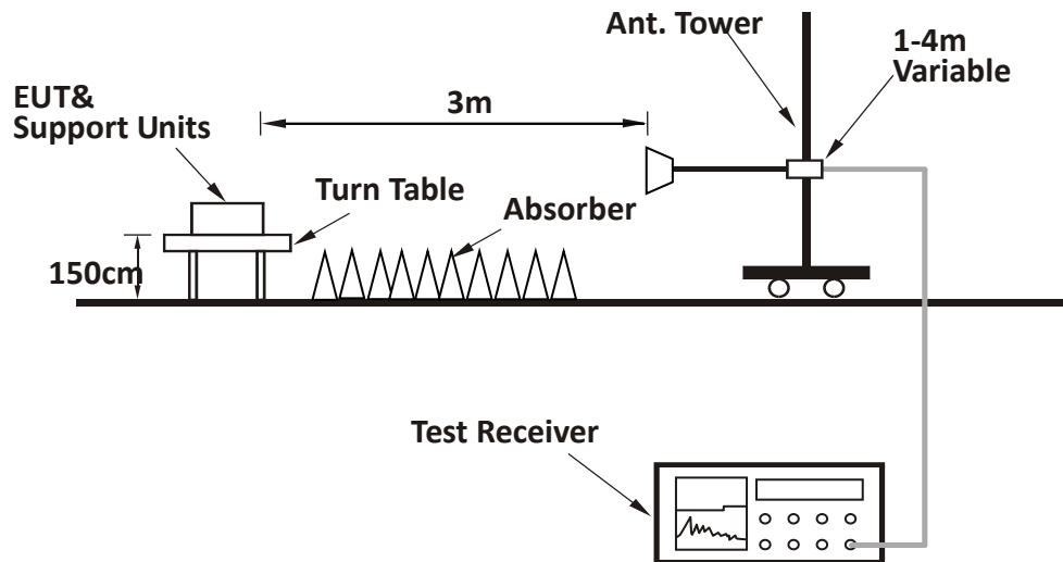
**TEST REPORT****7.4 Test Results of Radiated Emissions**
