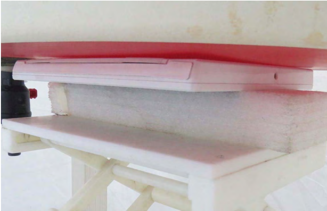
Picture 5: Back Side, the distance from handset to the bottom of the Phantom is 0mm
