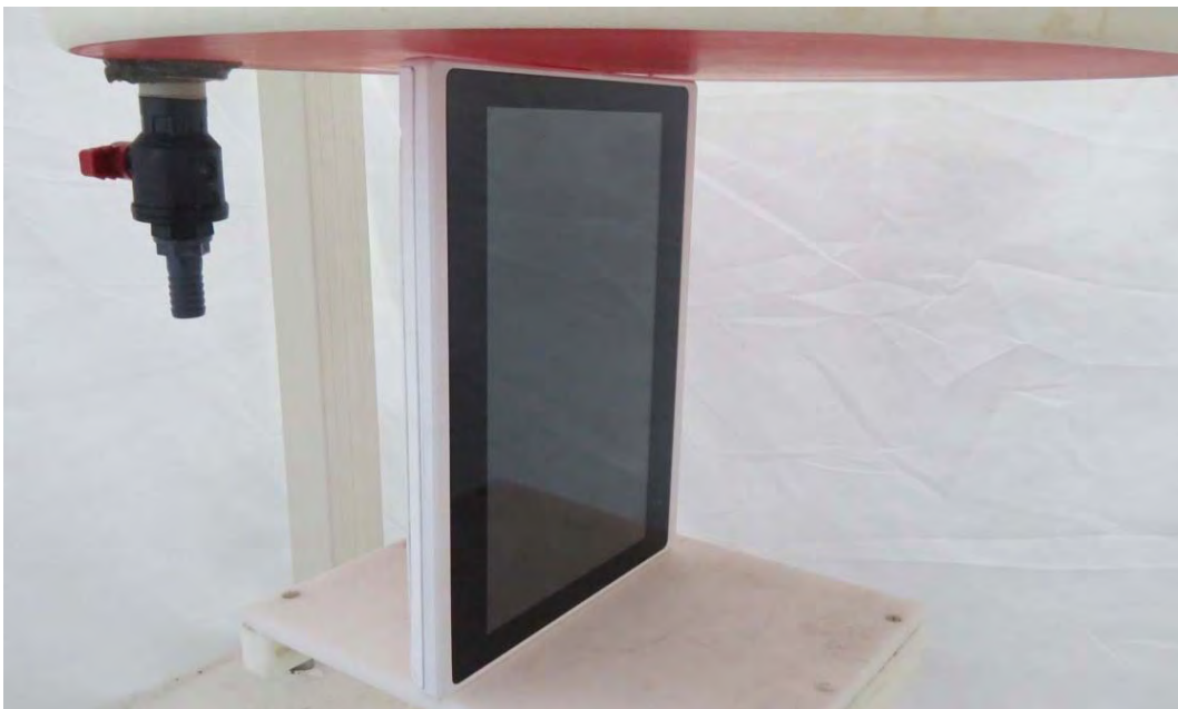
Picture 6: Left Side, the distance from handset to the bottom of the Phantom is 0mm
