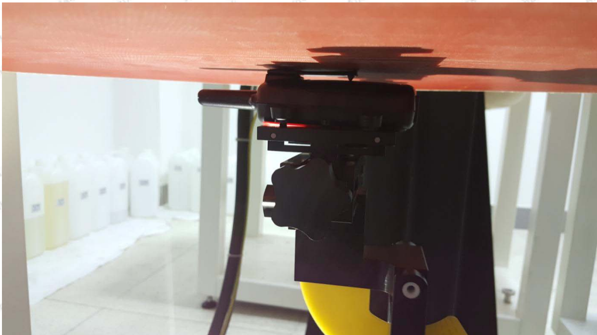
Body-worn, the front of the EUT towards ground (The distance was 0mm)
