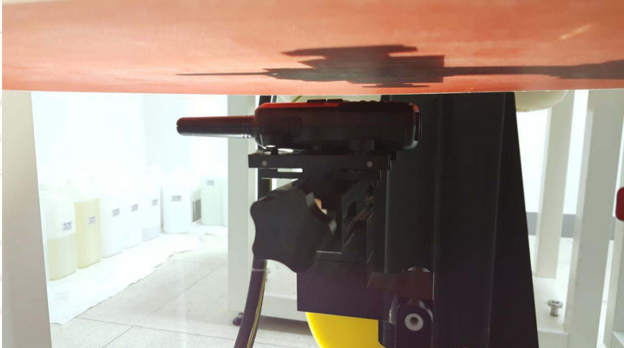
Face-held, the front of the EUT towards phantom (The distance was 25mm)
