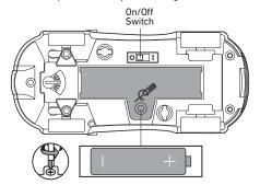
The remote requires 2 "AAA" 1.5V batteries (not included). Use tool to press the fastener and release the battery door for the remote.
