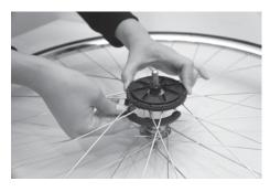
**4\_ Mounting Sub Disk**Place the sub disk on the opposite side of the main disk.
