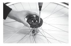
**5\_Fastening the Disk**Connect the main disk and sub disk, tighten them with 8 bolts.
