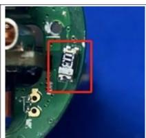
The antenna is Chip antenna. The best case gain of the antenna is 3 dBi.
