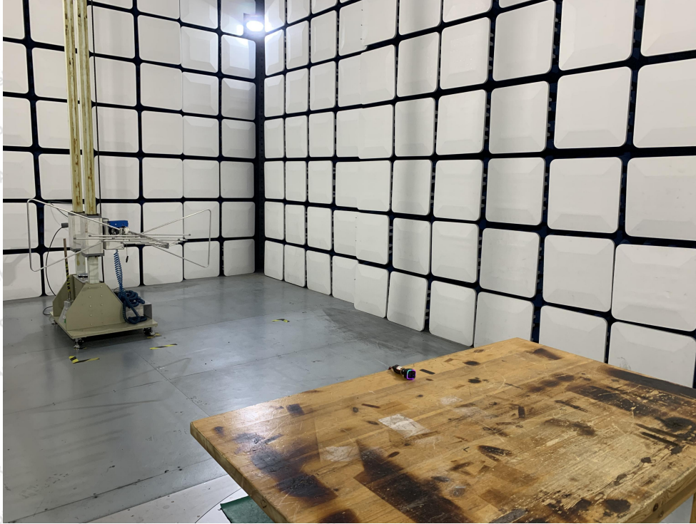
Photo of Radiation Emission Test
