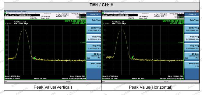
Note: When the PK measure result value is less than the AVG limit value, the AV measure result values test not applicable.
