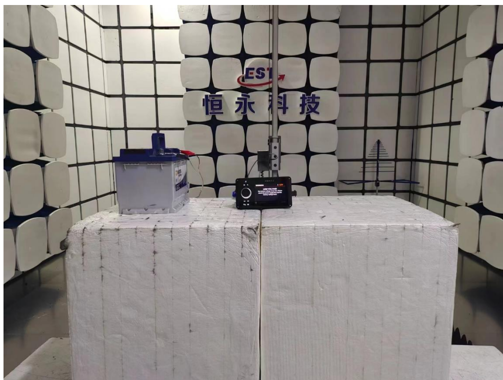
Radiated emission test: Above 1GHz
