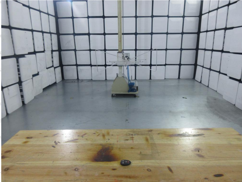
Photo of Radiation Emission Test
