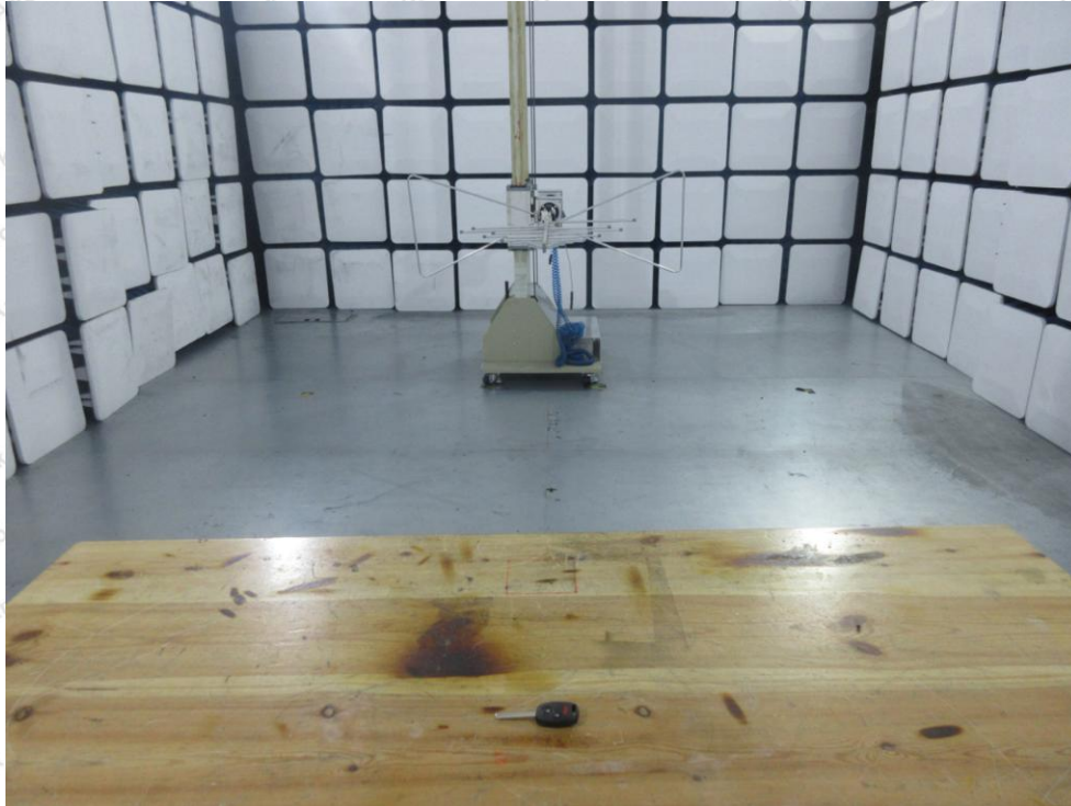
Photo of Radiation Emission Test
