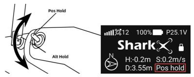
**Notice** when both joysticks are centered, if on **Pos Hold** mode, the drone will hover at the current position, and if on **Alt Hold** mode, the drone might get pushed away from the current position by wind.
