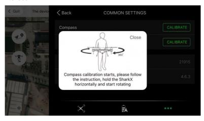
4.5.4. Following the audio instructions, hold the drone horizontally with its nose outwards and complete the horizontal calibration. And then hold the drone vertically with its nose downwards and complete the compass calibration.
