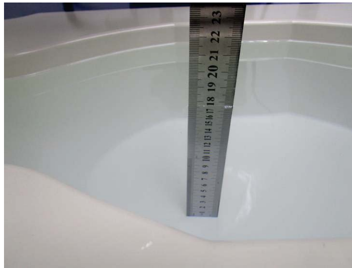
Liquid Height for Body SAR
