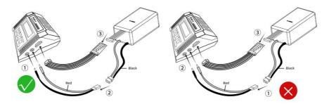
For safety concerns, please make sure the cables are connected with the adaptor first
