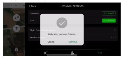
**Notice** if the SharkX appears forward or backward shift during flight, re-calibrate the compass. If problem still exists, contact local distributor/dealer and seek help.
