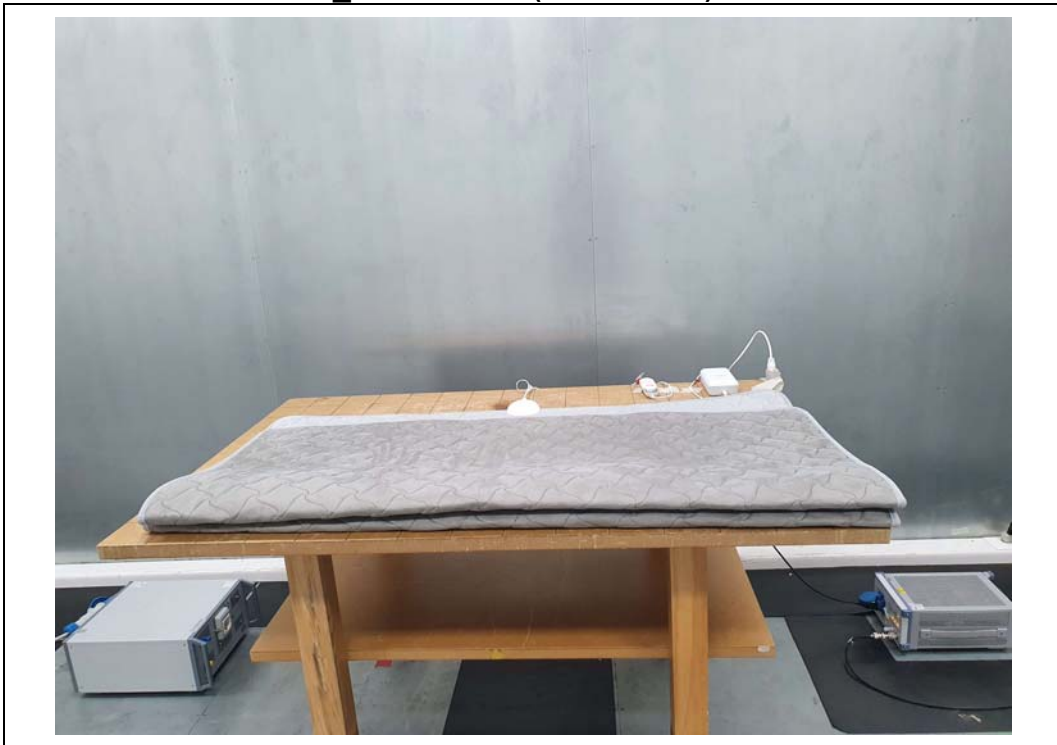
Conducted emission_Basic model (EME501-DP) Front
