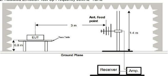
3. Radiated Emission Test-Up Frequency Above 1GHz
