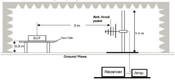
3. Radiated Emission Test-Up Frequency Above 1GHz
