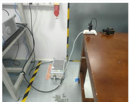
Conducted Emissions at AC Power Line (150kHz-30MHz)
