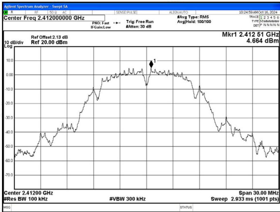
Tx. Spurious NVNT b 2412MHz Ant1 Emission
