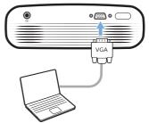
2 On your computer, adjust the screen resolution of the computer to the correct setting and switch the VGA signal to an external monitor. The following resolutions are supported:
