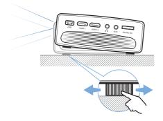
3 To adjust image focus, turn the focus knob on the top of the projector.
