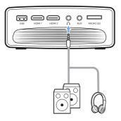
2 When connecting to the headphones, use the volume control on the remote control to adjust the volume to a comfortable level.
