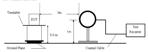
Figure 1. 9KHz to 30MHz radiated emissions test configuration
