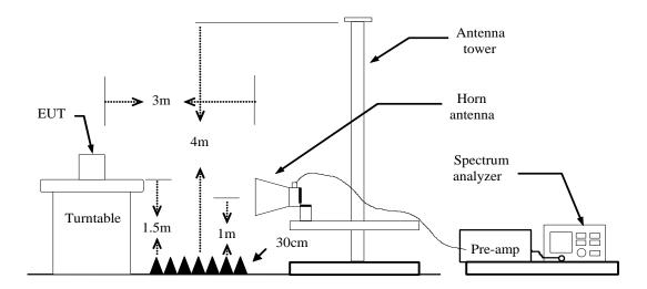
Figure 3. Above 1GHz radiated emissions test configuration
