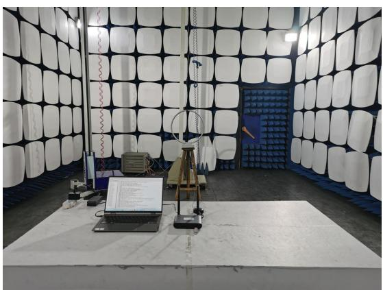
3. Radiated emission (9KHz-30MHz)
