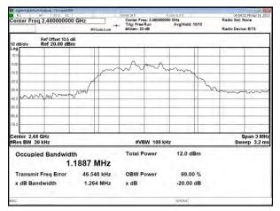
Cerpass Technology Corp. D-FD-507-0 V1.1 Page No. :50 of 61 Modulation Type: 8DPSK (3Mbps)
