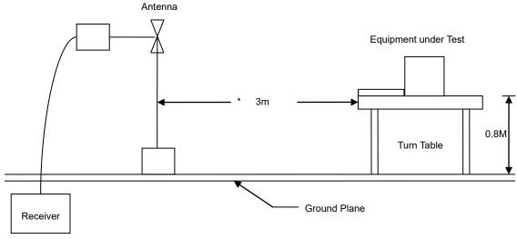
Above 1GHz Test Setup
