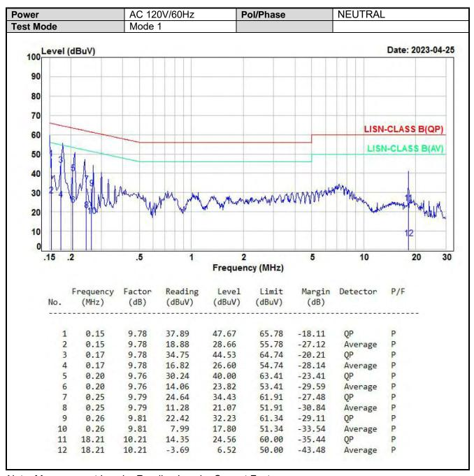
Note: Measurement Level = Reading Level + Correct Factor
