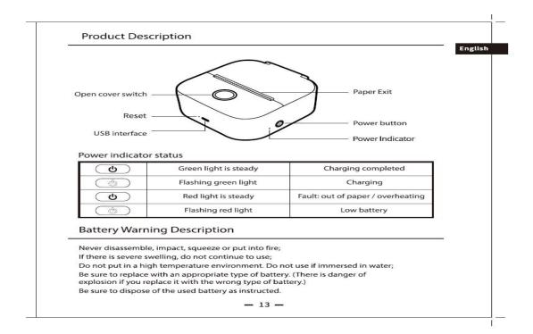
Product Description Open cover switch Reset USB interface Paper Exit Power button Power Indicator
