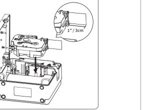
English Install the tape and pull out a section of the label about 1" (3cm) from the paper outlet.
