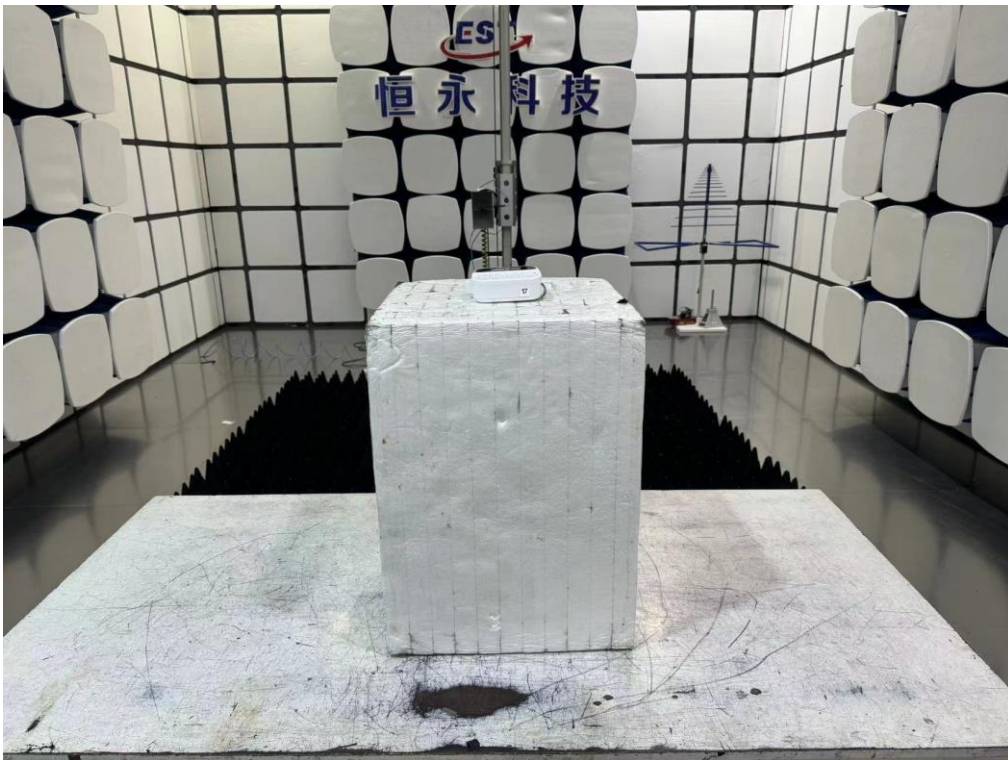
Radiated emission test: Above 1GHz
