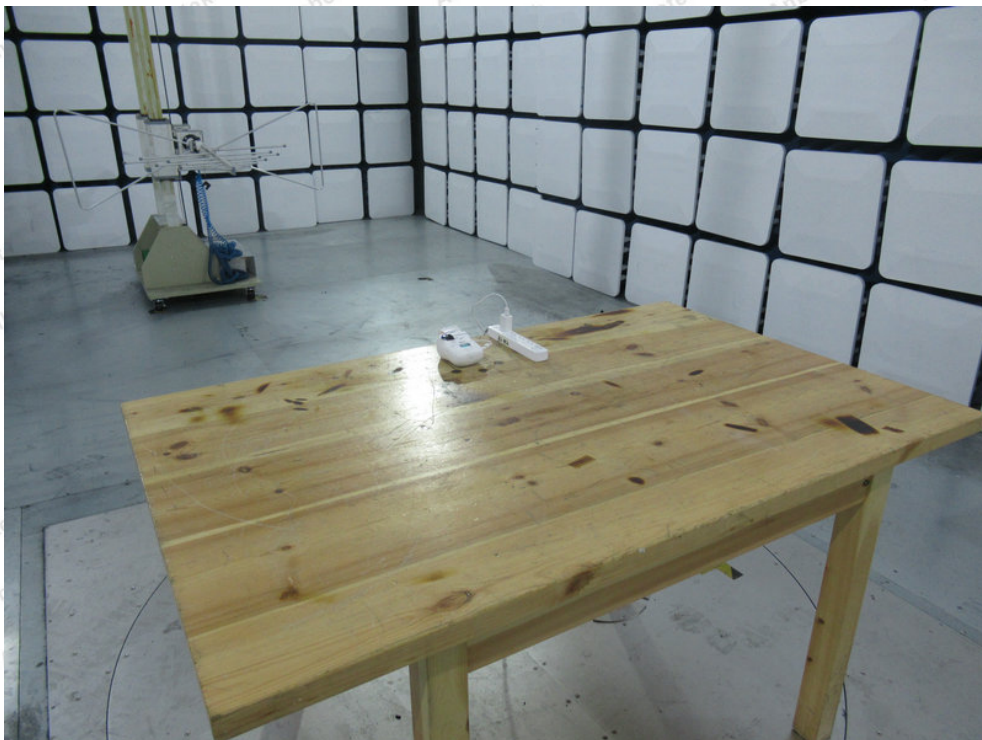
Photo of Radiation Emission Test
