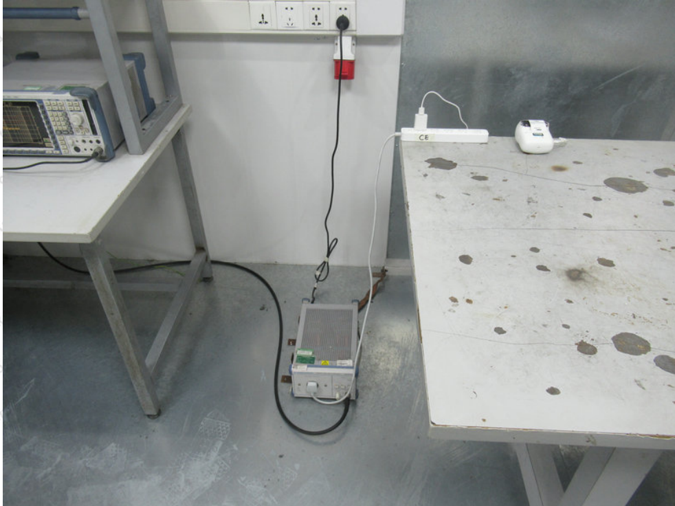
Photo of Conducted Emission Measurement
