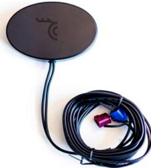
Install the Cellular-GNSS-Antenna on the dashboard or on the windshield or on the dashboard below using the fastening pad. It is also possible to install more firmly on a mounting plate as long as the plate is not made of metal. Run the cable to the Cloud-Boxx and insert the blue and purple connectors. Roll up any extra cable and fasten it with some zipties. Make sure airbag functionality is not compromised. The antenna must be mounted so that the Hirschmann logo is directed skyward.
