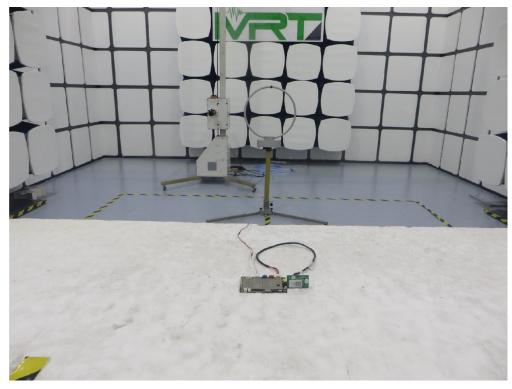
Description: Radiated Spurious Emission Test Setup for above 30MHz
