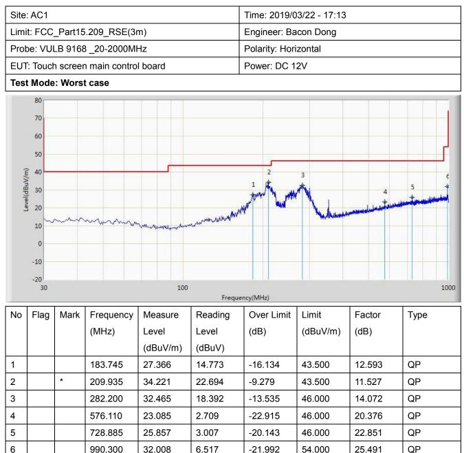
Note 1: Measure Level ( $dB\mu V/m$ ) = Reading Level ( $dB\mu V$ ) + Factor (dB)
