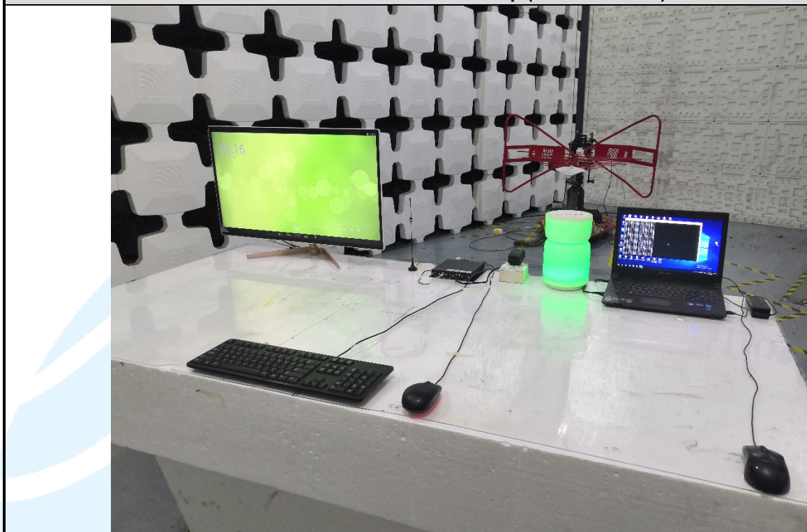
Radiated emission Test Setup (30 MHz~1 GHz)
