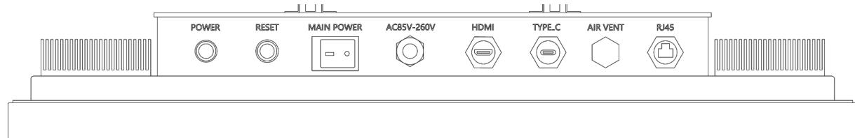
Insert the USB TYPE C cable into the port labeled TYPE\_C, after taking off the lid. Please use as the minimum a shielded IP54 cable for the connection.
