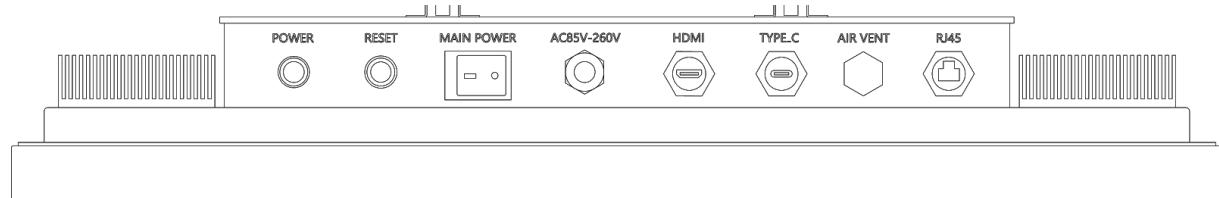
Insert the cable into the port labeled as HDMI, after taking off the lid. Please use as a minimum a shielded IP54 cable for the connection.
