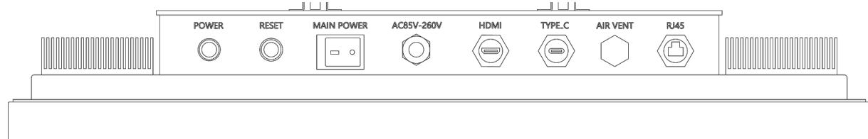
Insert an RJ45 cable into the ETHERNET port labeled with RJ45, after taking off the lid. Please use only a Cat7 (shielded twist pair Type) cable for the connection. (10/100 Mbps)
