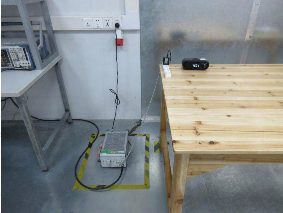
Photo of Power Line Conducted Emission Test
