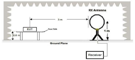
(2) Radiated Emission Test-Up Frequency 30MHz~1GHz
