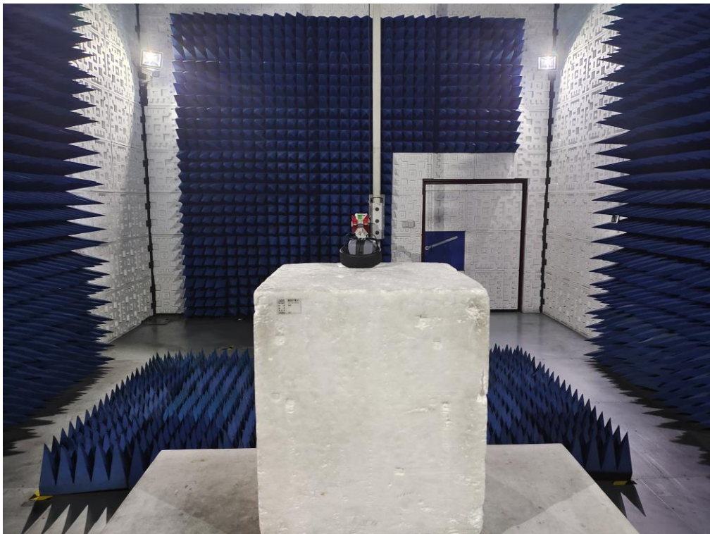
RADIATED EMISSION TEST SETUP ABOVE 1GHz
