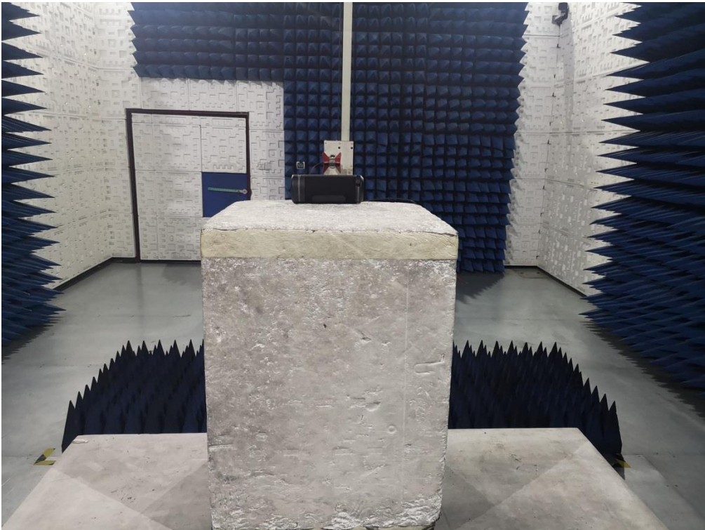
RADIATED EMISSION TEST SETUP ABOVE 1GHz
