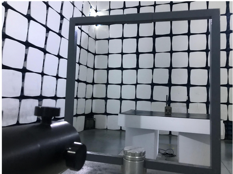
Radiation Emission Test Setup (Below 30MHz)
