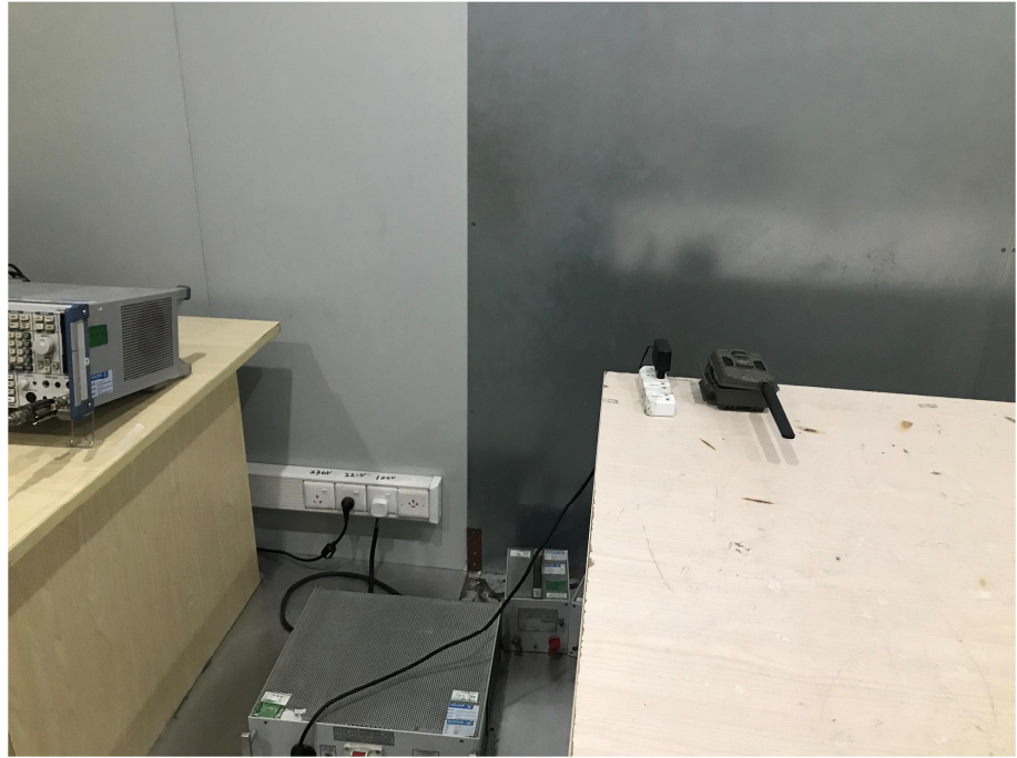
Conducted Emission Test Setup*
