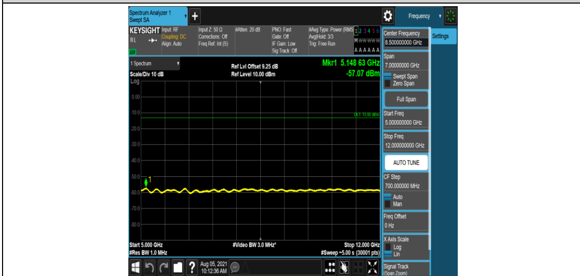
Band4-10MHz-16QAM-20350-1-0-High-5000-12000--57.07-PASS
