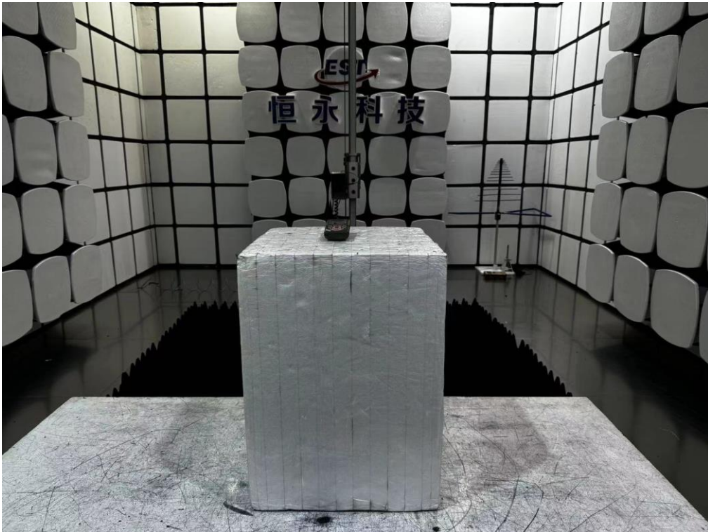
Radiated emission test: Above 1GHz
