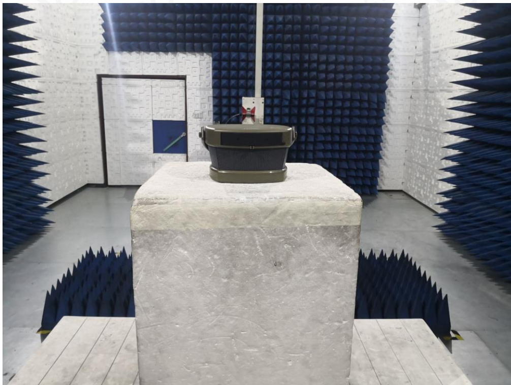
RADIATED EMISSION TEST SETUP ABOVE 1GHZ
