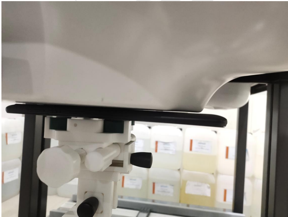
Body Back side(separation distance is 0mm)
