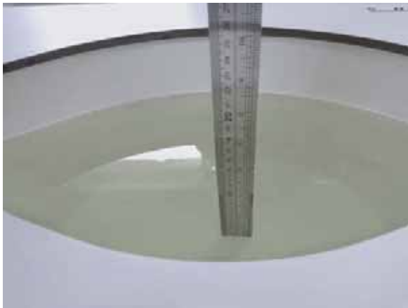
Liquid depth in the head phantom (2450MHz)
