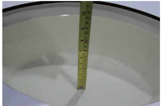
Liquid depth in the body phantom (5GHz)
