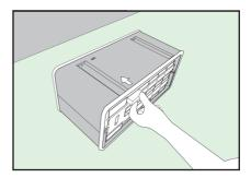
• Remove packs by pulling out from the bottom opening of each section as per the visual shown opposite.
