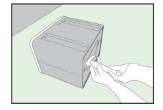
Turn unit on by plugging in or stacking on top of an already powered POS unit.
