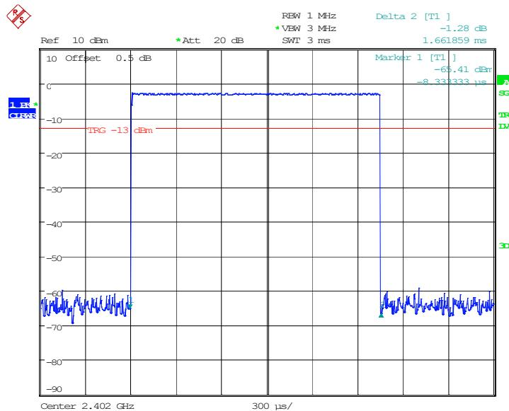
**BDR (GFSK): Pulse time, Middle Channel, DH3**
