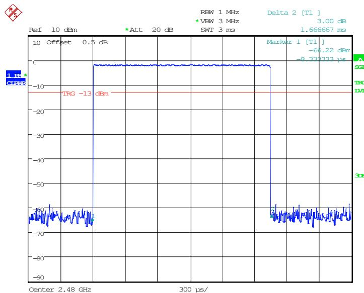
**BDR (GFSK): Pulse time, Low Channel, DH5**
