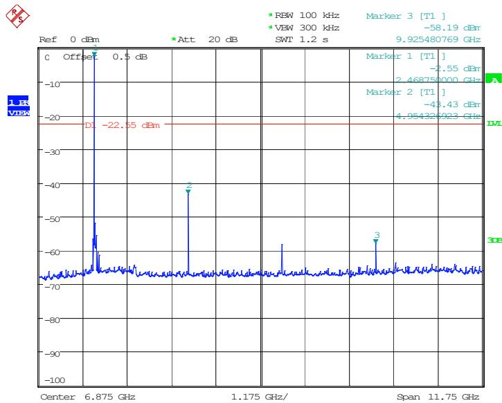
**EDR ( $\pi/4$ -DQPSK): Low Channel**
