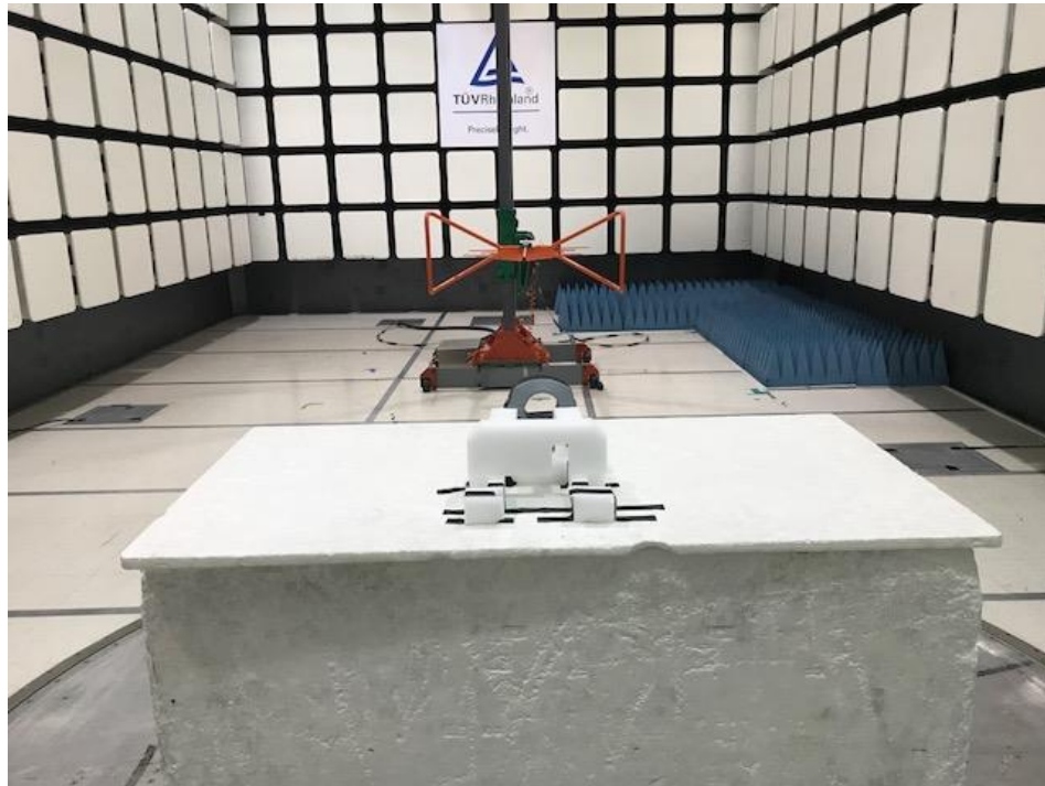
Figure 5: Test Setup for 30 MHz to 1 GHz (Rear View)
