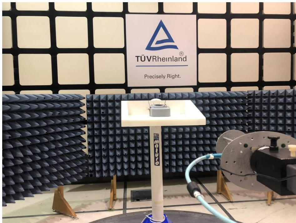
Figure 10: Test Setup for 1 GHz to 40 GHz (Front View)
