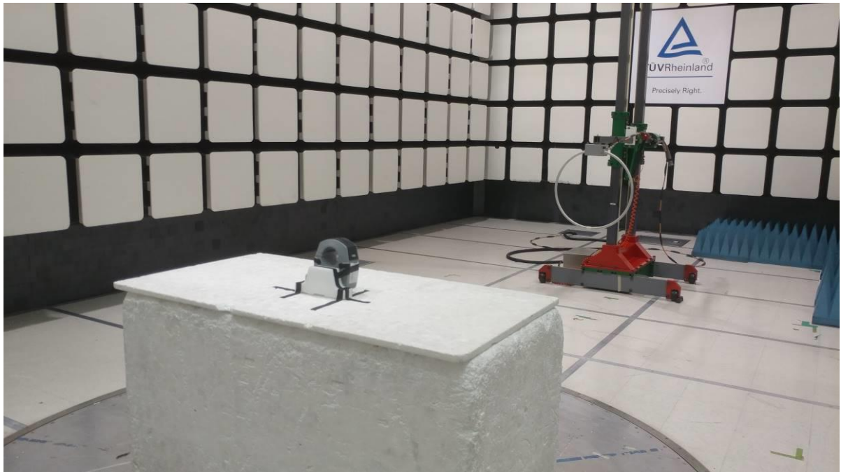
Figure 3: Test Setup for 9kHz to 30 MHz (Rear View – Antenna 0°)
