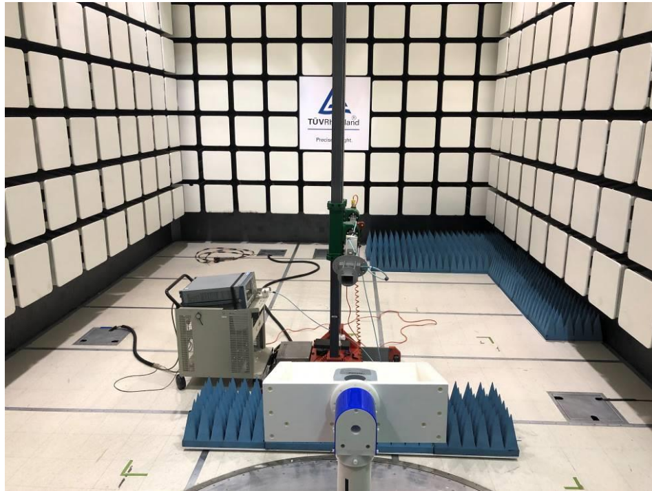
Figure 9: Test Setup for 18 GHz to 40 GHz (Rear View)
