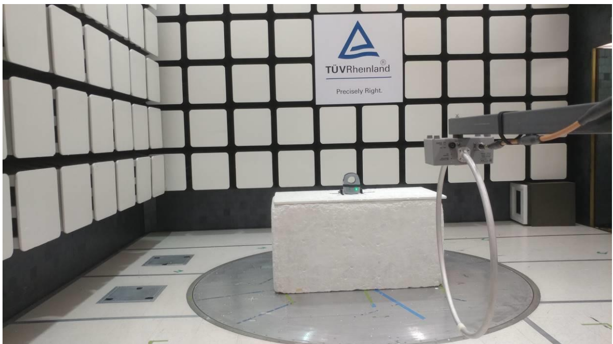
Figure 4: Test Setup for 9kHz to 30 MHz (Front View – Antenna 90°)
