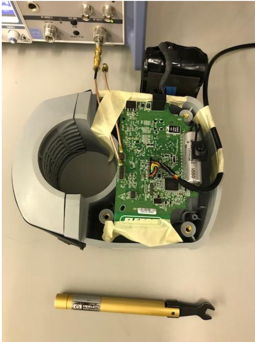
Figure 2: Test Setup for conducted measurements at internal u.fl connector - detail
