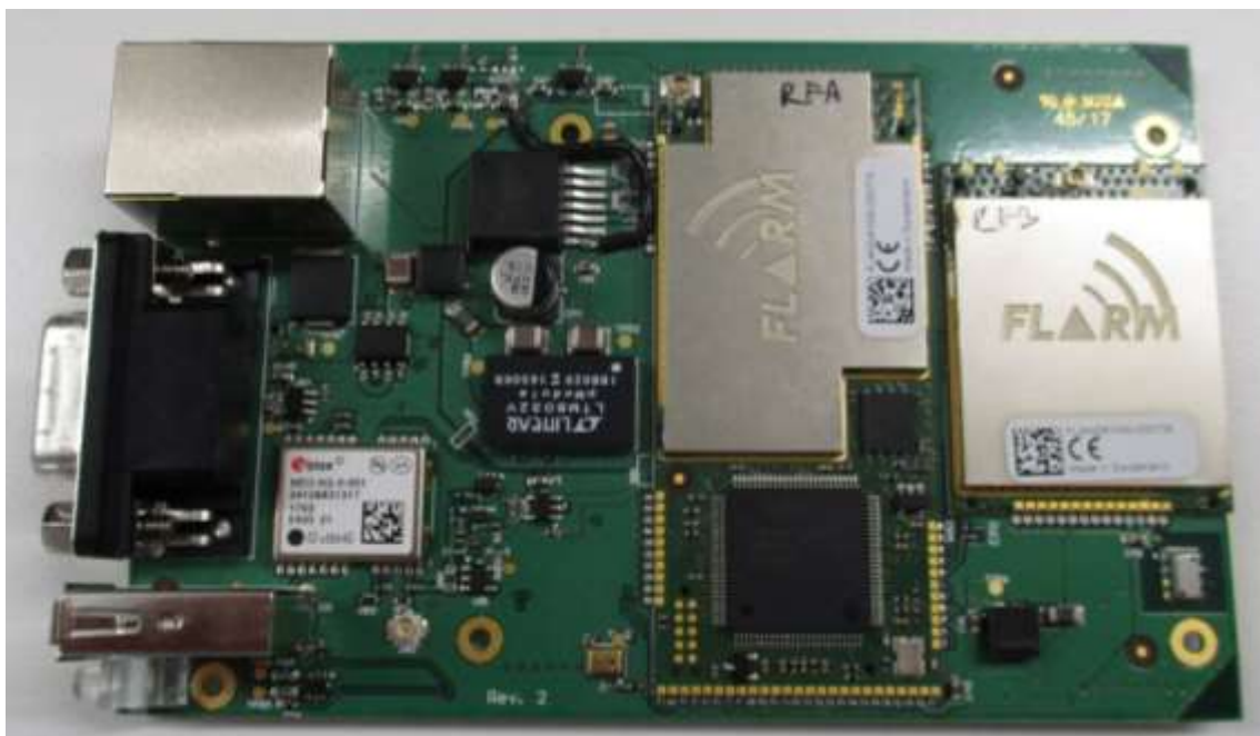
Figure 9: Photo of host ( LXNAV Application module evaluation board ) with modules, top side
