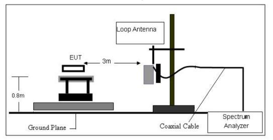
(B) Radiated Emission Test-Up Frequency 30MHz~1GHz
