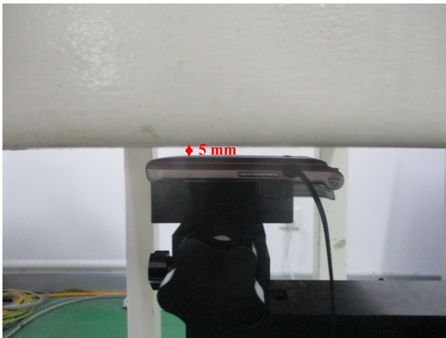
Body Worn Back Setup Photo (5mm)
