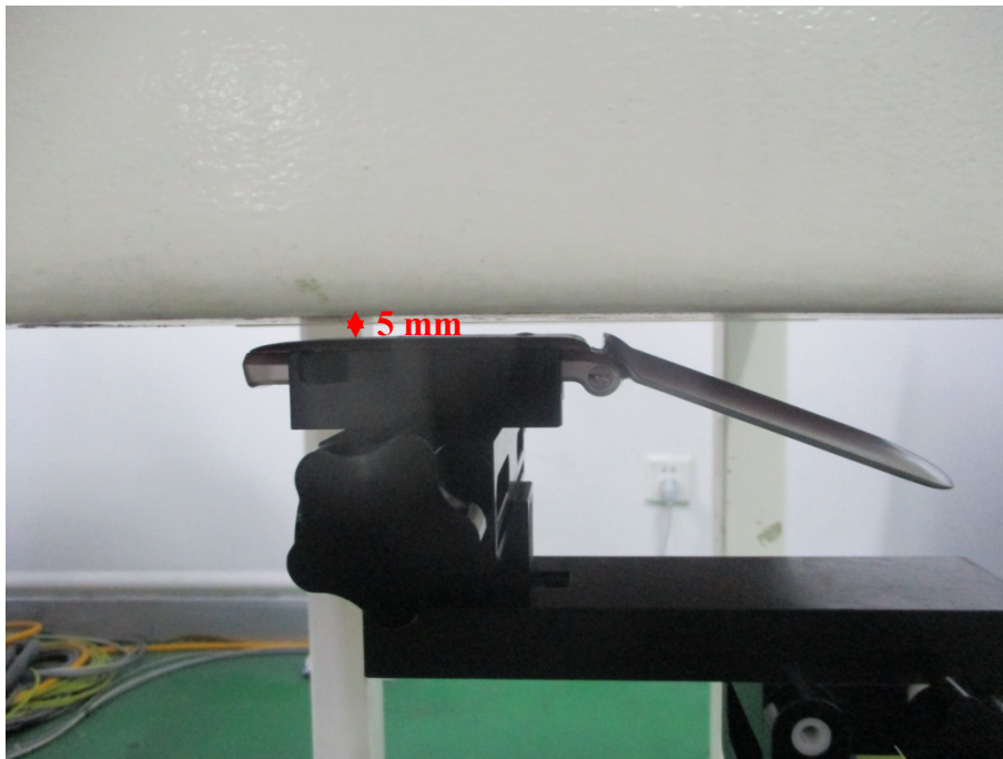
Body Worn Back Setup Photo (5mm)
